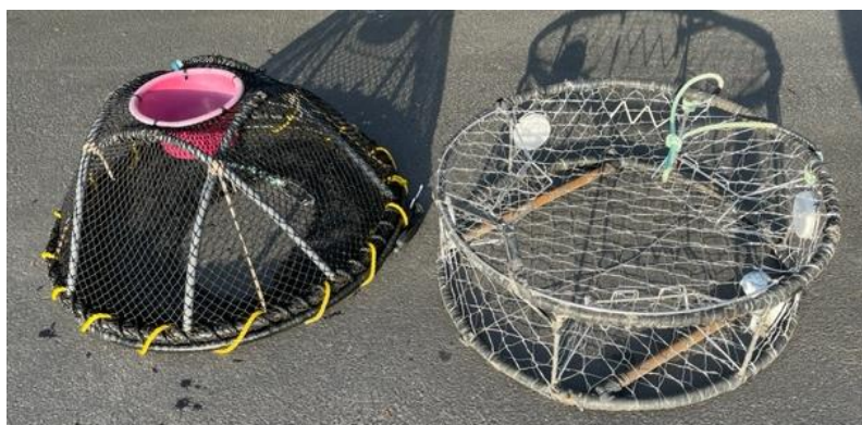
Figure 1. The two trap styles used: cone style (left) and commercial style (right).
