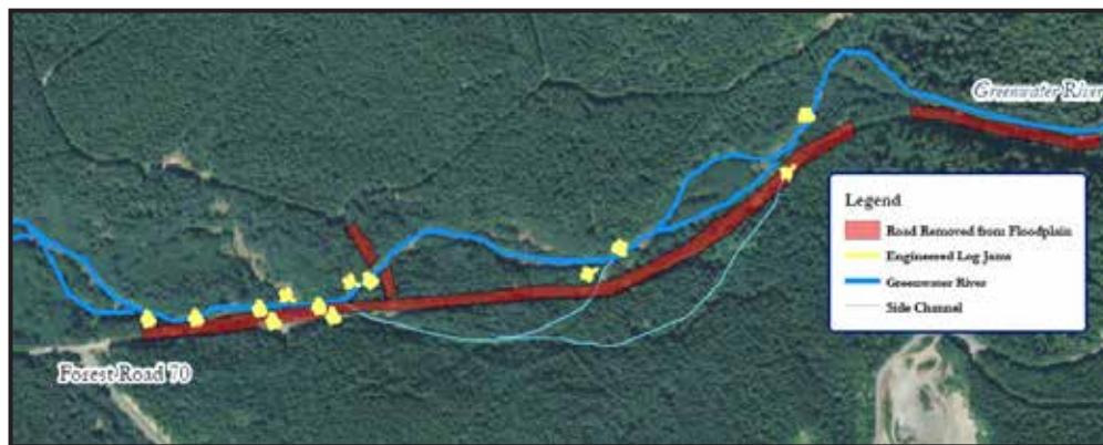
Restoration Plan for the Greenwater River Floodplain Restoration Project, including placement of 13 ELJs and removal of nearly 1-mile of abandoned Forest Road from the floodplain
